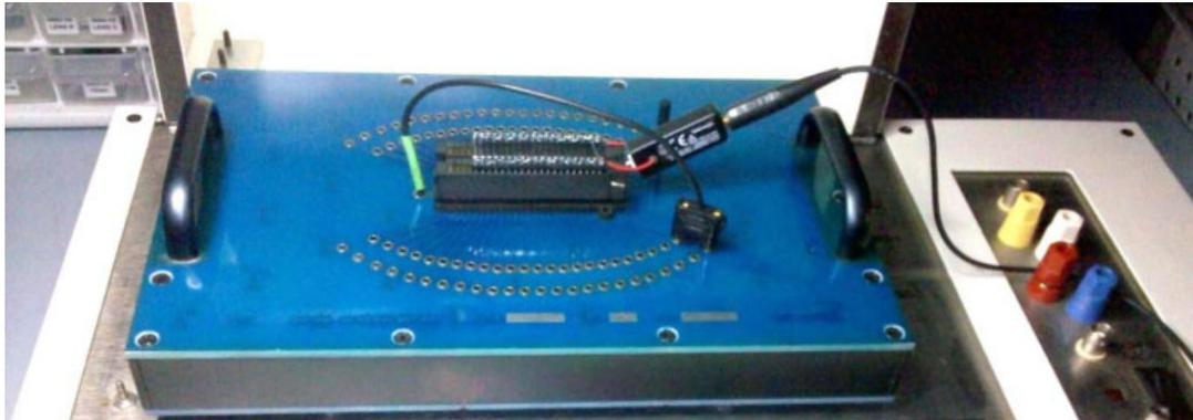
*Figure 6: HBM Tester being Evaluated for Low Parasitics*
