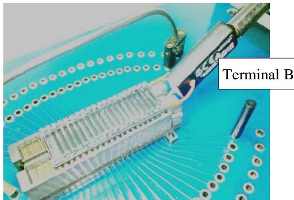
*Figure 7: 40 Pin DIP Shorting Test Device with the Current Probe Connected between the Unconnected Pin 1 and Group Connected Pin 40*
