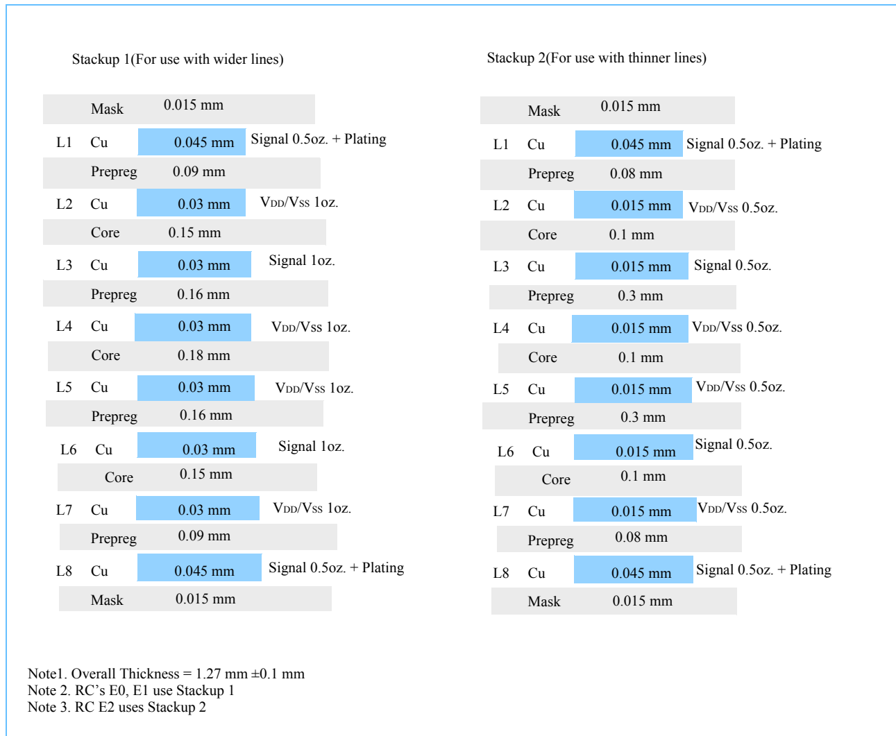
Figure 44 — Eight-Layer Stackup (Example)
